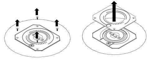
2. Using a screwdriver, remove the housing assembly. Clean the assembly especially on the bushing – bollard surfaces.
