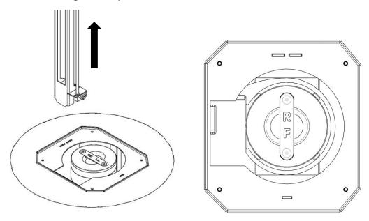
4. Remove the bollard assembly and lay it on the side to remove the rope from the bollard. Tie the loose ends of the rope together and secure it to prevent it from falling in.
