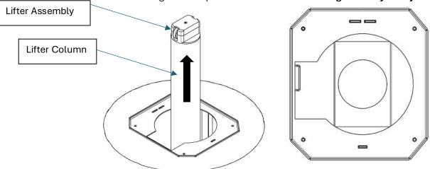
6. Clean out the interior of the bollard shell with a pressure washer, and vacuum out the debris if drainage is not working. **Note:** The proper position of the bollard pad.
