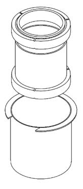
Casing assembly consists of 2 bushings and one support
