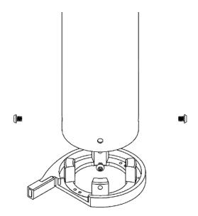
Bollard is attached to lifter with 4 button head screws
