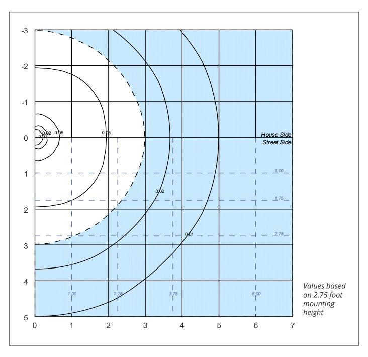
The isofootcandle values shown in the plot above are based on a mounting height of h = 2.8 feet. Grid values show multiples of mounting height. The isoilluminance contour lines are expressed in units of footcandles. The values expressed are based on the direct light from a single unit without the contribution of room reflections.
