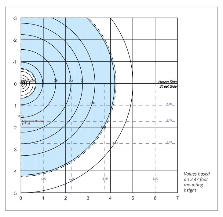
The isofootcandle values shown in the plot above are based on a mounting height of h = 2.5 feet. Grid values show multiples of mounting height. The isoilluminance contour lines are expressed in units of footcandles. The values expressed are based on the direct light from a single unit without the contribution of room reflections.
