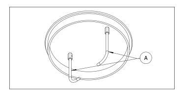
**STEP 7:** Fit the cap onto the bollard, ensuring that the longer axis of the cap aligns with the long axis of the bollard base. Press the cap and the J-anchors into the wet concrete until the cap sits flat on the base.
