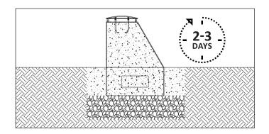
**STEP 9:** Inspect the installation. The vertical side of each bollard should be perpendicular to the surface of the concrete. The sloped side of the Martello Bollard's body should face the road. If placed at a corner, the sloped side should face the center of the corner.
