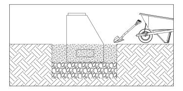
**STEP 5:** When the concrete fills the installation hole, begin filling the body of the bollard through the holes at the top. Continue to pour until the wet concrete fills the base of the bollard to within 1/2" of the top.
